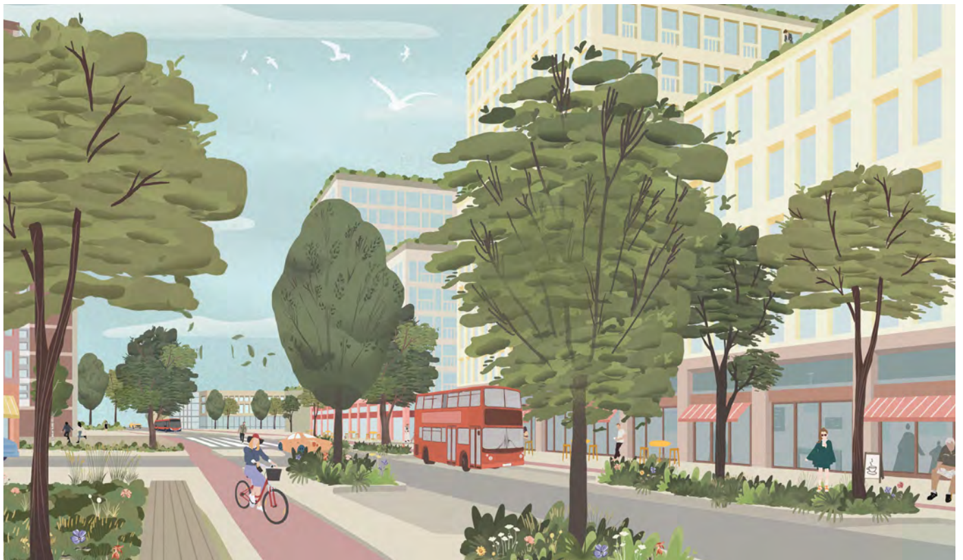
Fig. 118. Recharacterise the ring road as an urban street, creating active frontages, spaces for cyclists, pedestrians, buses and cars, new at-grade crossings and on-street parking formalised along tree planting
